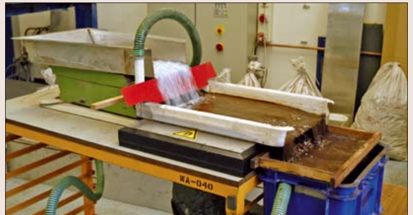
This test set-up devised by doctoral student Erwin Bakker was used for separating shredded PET from contaminants such as grit, glass, and metals. This test set-up also uses a magnetic fluid, but this time the fluid moves along with the PET particles. The contaminants remain behind at the bottom of the container. The PET particles are extracted by a screen.
