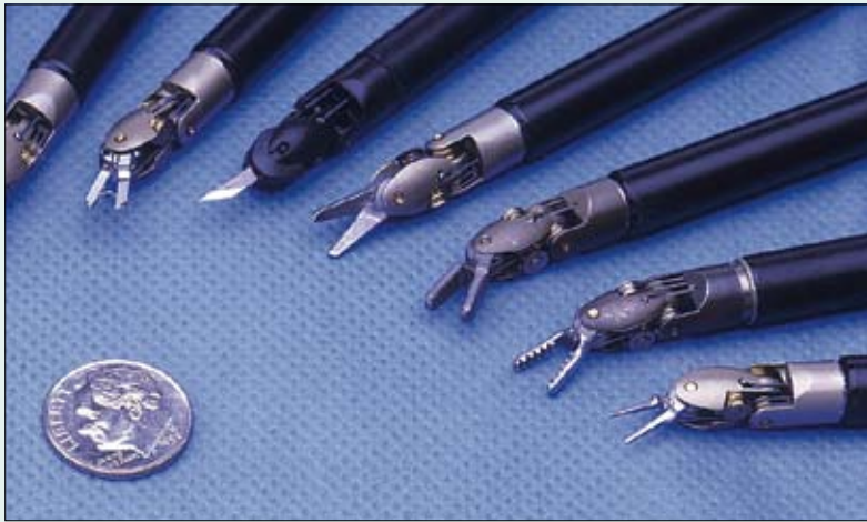
The tools of the robot made by Intuitive Surgical Inc. are fairly complex and require an expensive sterilisation technique.
