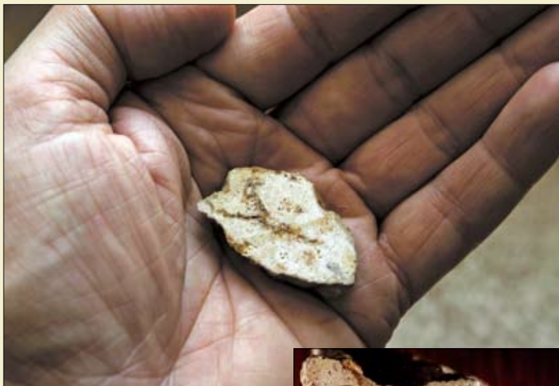
A section through the Cheops limestone sample used for tests using electron microscopy and thin section techniques.
