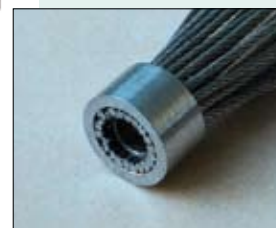
Cross-section of the tip of the recently developed third prototype of the Endo-Periscope, showing the ring of cables, surrounded by two helical springs and fixed at the tip between two rings.
