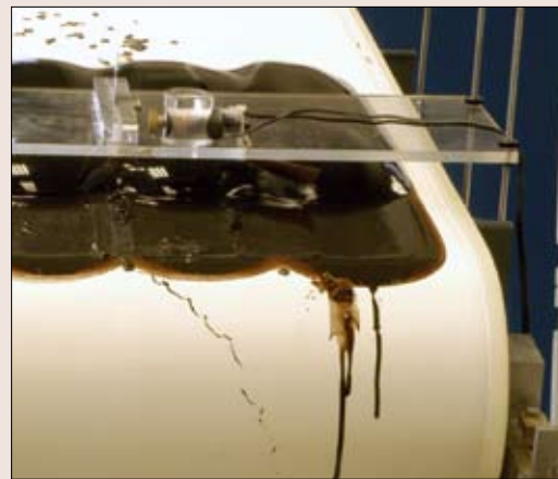
The metal particles are extracted in two flows, one in the centre, and one along the edge.
