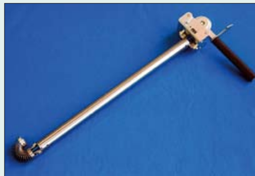
Dr Ir. Paul Breedveld and Professor Shigeo Hirose of the Tokyo Institute of Technology, invented the Ring Spring consisting of spring steel discs spot-welded together. The Ring Spring has an asymmetrical bending stiffness and a very high torsion stiffness. The holes conduct the wires that control the tip.
