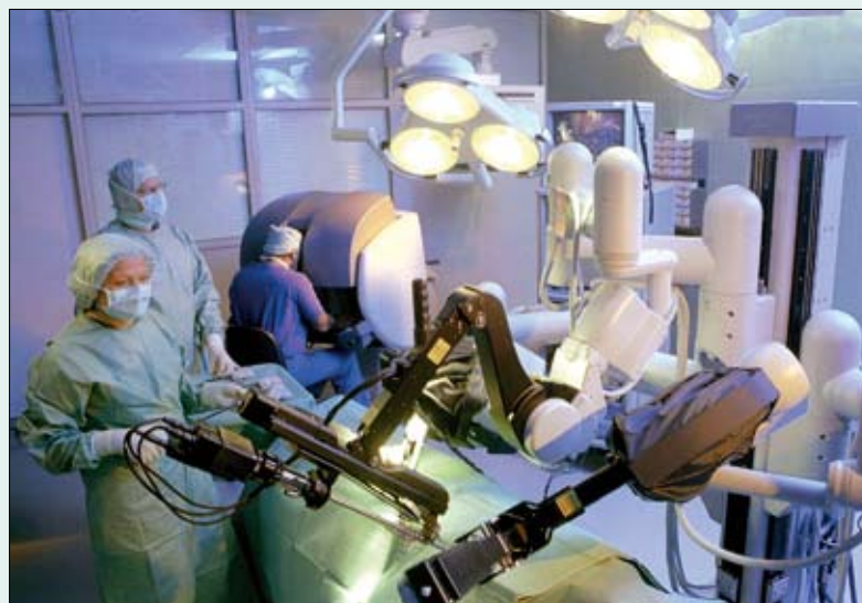
Modern telemanipulators, such as the Da Vinci by the American firm Intuitive Surgical, use remotely controlled steerable instruments. Such instruments are fairly complex and difficult to miniaturise.
