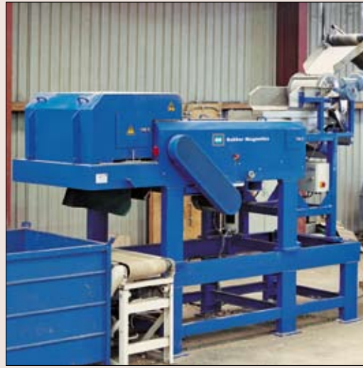
Eddy current separator used for separating aluminium from PET waste. It uses a rapidly changing magnetic field to eject the aluminium particles from the mixture.
