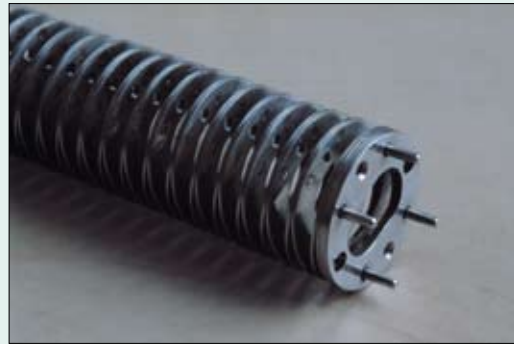
Dr Ir. Paul Breedveld and Professor Shigeo Hirose of the Tokyo Institute of Technology, invented the Ring Spring consisting of spring steel discs spot-welded together. The Ring Spring has an asymmetrical bending stiffness and a very high torsion stiffness. The holes conduct the wires that control the tip.
