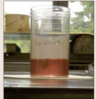
If a lump of magnesium (density approx. 1700 \text{ kg/m}^3 ) is dropped into a manganese chloride solution (density approx. 1400 \text{ kg/m}^3 ), it sinks to the bottom. If the container holding the solution and the metal is then placed on a magnet, the metal will rise in the solution (picture on the right) because of the increased density of the fluid.
