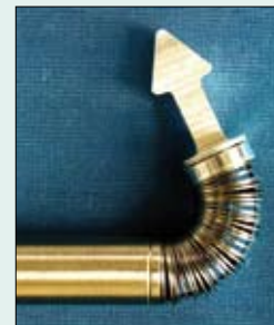
The tip of the second prototype can be steered over 120° in all directions.
